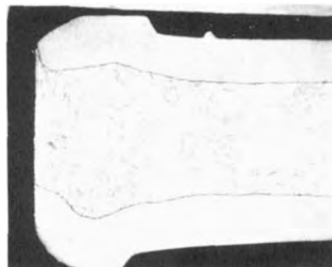
Fig. 3 Metallographic cross section of the edge of a cupronickel-clad copper coin
